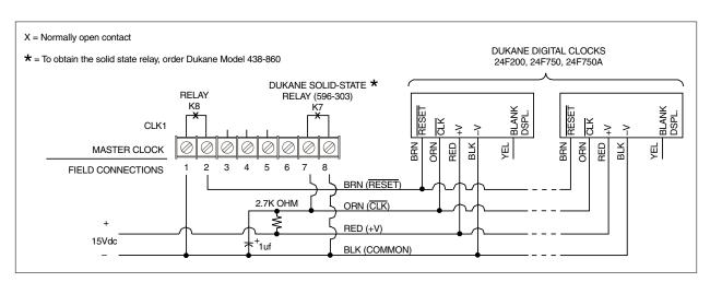
Figure B-8 Wiring Dukane 24F200, 24F750, and 24F750A Digital Clocks for 15Vdc
